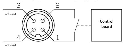
Only contacts 1 and 2 are used, which are closed at the right moments with a relay. The maximum switching current is not more than 1.5A; the maximum switching voltage is not more than 22oV. At the moment when the source is supposed to be running, the relay contacts are closed, when the source is supposed to be off – they are open.
